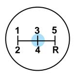
You can shift into R (Reverse) only by moving the gearshift lever from left of 3 (Third) and 4 (Fourth) gears before you shift into R (Reverse). This is a special lockout feature which prevents you from shifting into R (Reverse) when you downshift from 5 (Fifth).
